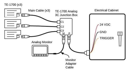
**Note:** When connecting the monitor to the junction box, the 5m monitor extension cable must be used. This cable, which converts the monitor's aviation style connector to the Mil-spec connector that mates into the junction box, comes standard with the ExcelSense analog monitor.
