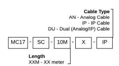
Main cable can be used in all ToughEye-1700 installations. The analog cable includes a 75-ohm coaxial cable for CVBS transmission. The IP cable includes a shielded Cat-5e cable for 10/100 Base-T signal transmission.
